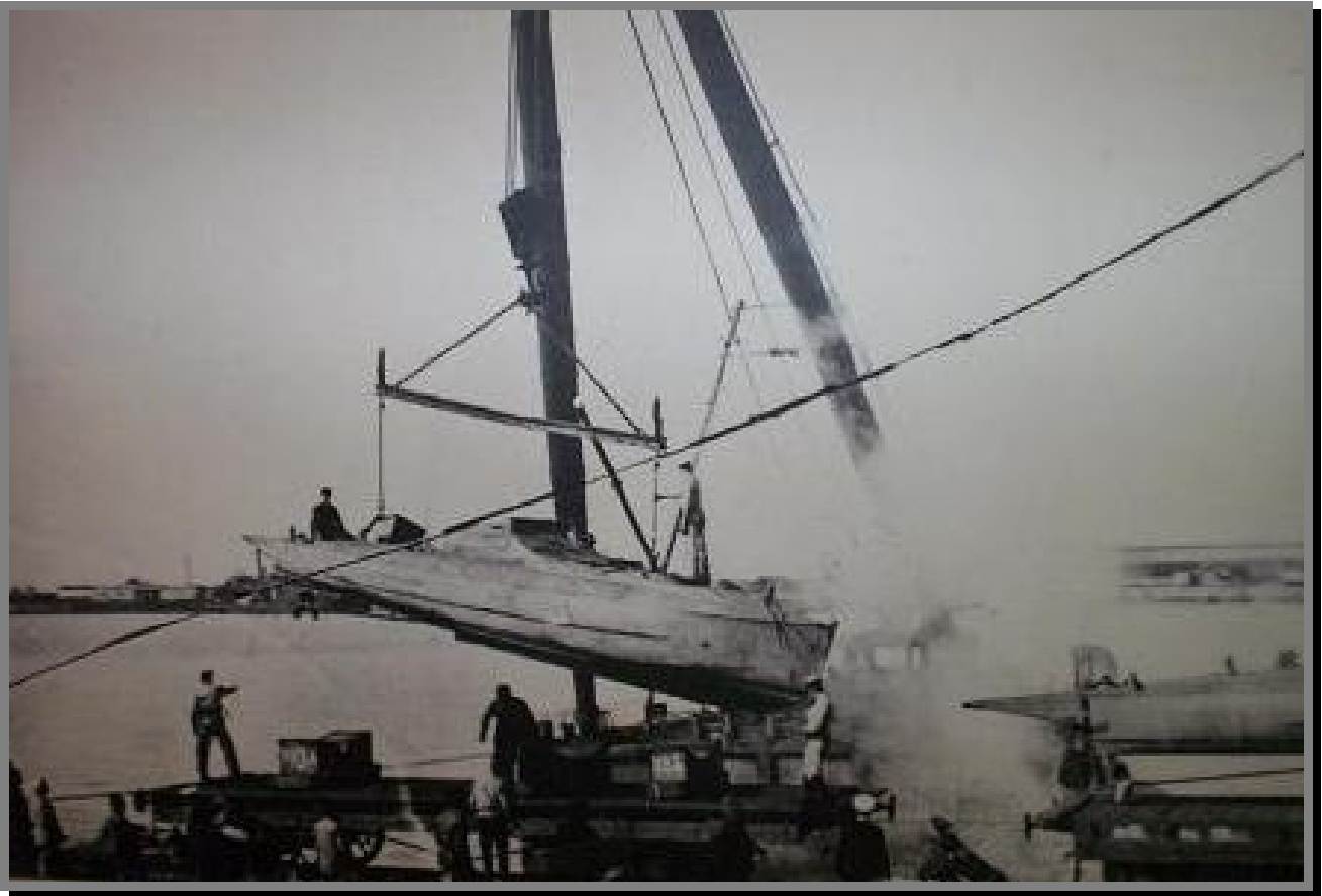
CMB61 is lifted onto a railway truck for transport overland from Batum on the Black Sea to Baku on the Caspian.
